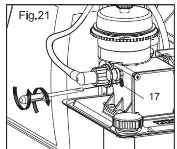
When the adjustment is correct the engine pulse note is regular and no flame appears at the resonator end.
