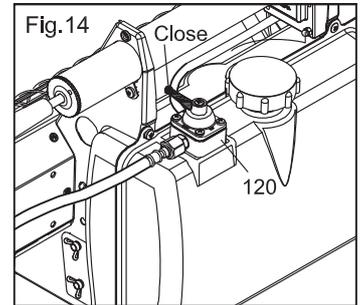
Normally emergency cut-off device fitted on E models will automatically prevent the solution being injected when fogger is not operating.
