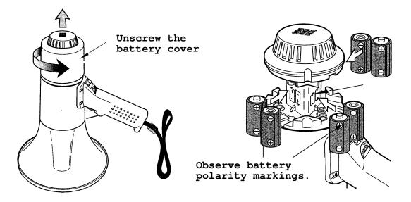
Unscrew the battery compartment cover, located at the microphone end of **PATROL**; turn the cover to the left (anti-clockwise) to remove it. Place six 'C' dry cells in the compartment as indicated, matching the polarity markings on the cells with those on the compartment. Replace the battery cover by turning to the right (clockwise).
